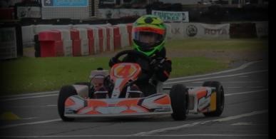
The K1 Stars kart is a fully blown MSUK regulated race chassis fitted with an adjustable seat and pedals. Powered by a Comer C50 Bambino engine, karts are capable of reaching a top speed of 35mph enabling our drivers a real taste of what it feels like to be behind the wheel of a racing machine. For extra safety measures, the latest fleet have also been fitted with a wrap around system to avoid wheel-to-wheel contact.
